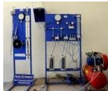
Fig. 2: Tri-axial Shear Test Setup
